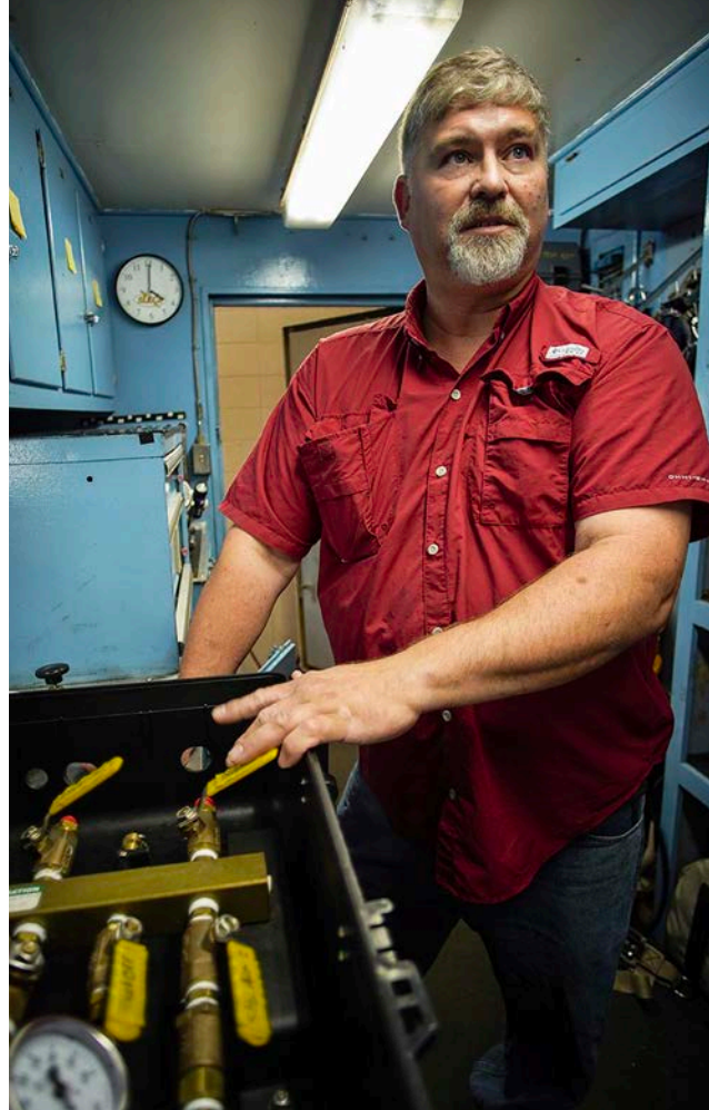
MIXOLOGIST Jerry Shepherd, head instructor at the South Louisiana Community College dive school, shows off a diving manifold, a system of valves that mixes the gases a sat diver would breathe during a dive.
