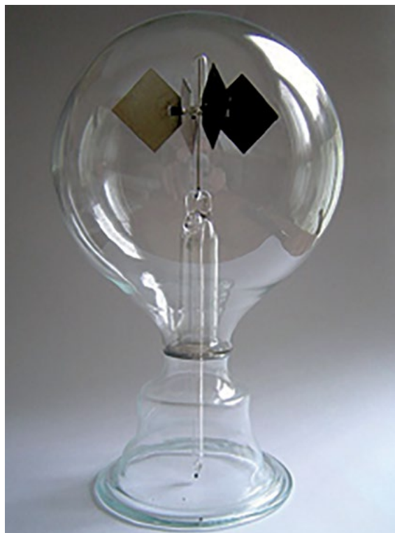
SPIRITS IN THE LIGHT In the 1870s, to investigate psychic forces, chemist William Crookes invented the radiometer (above), in which delicate vanes rotate when illuminated by light.
