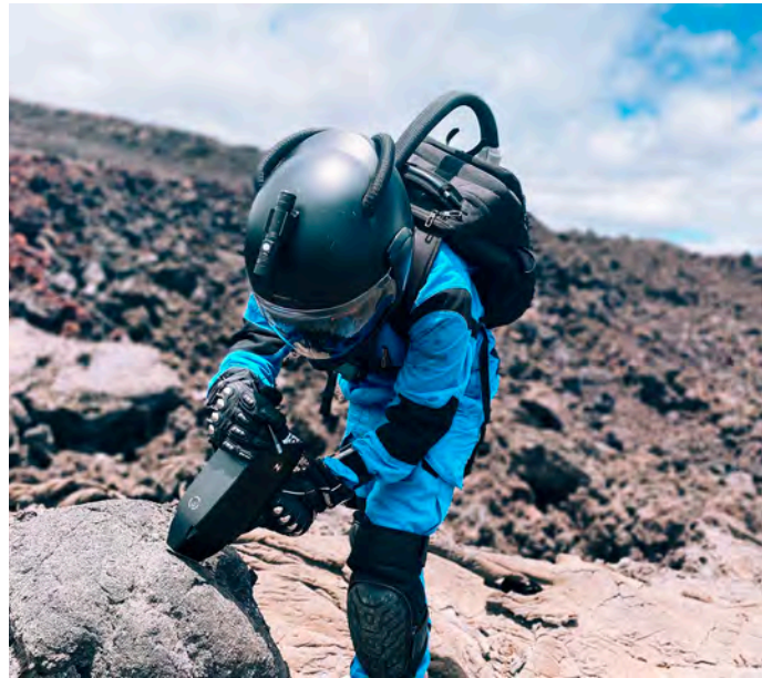
INTREPID EXPLORER Sarafina El-Badry Nance using the SciAps Laser Induced Breakdown Spectrometer (LIBS) while on "Mars" to analyze the elemental abundances of volcanic rocks.
