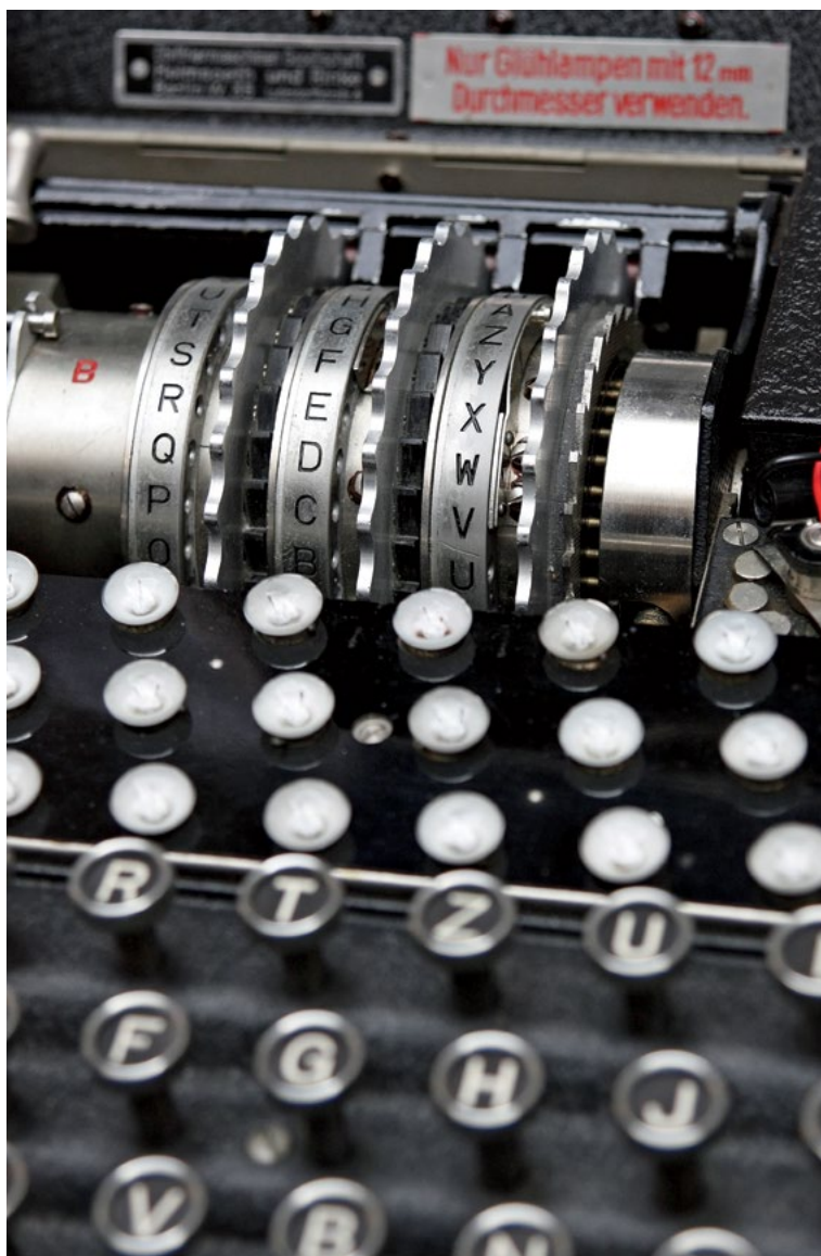
THE ENIGMA MACHINE: Used by Germany during WWII to encrypt and decrypt messages. Every time a key is pushed, the rotors turn to display a different letter.
